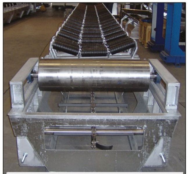
PULITORE a catena centrale forgiata (sotto) Cleaner with forged centre chain (bottom)
